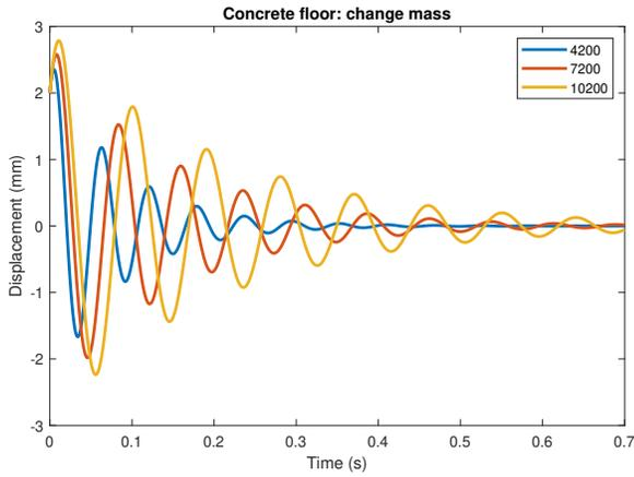
**Figure 2: Changing the density (mass) of the concrete floor. The legend is the mass (kg) of each floor.**
