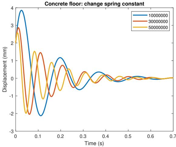
**Figure 3: Changing the spring constant of the concrete floor. The legend is the spring constant.**
