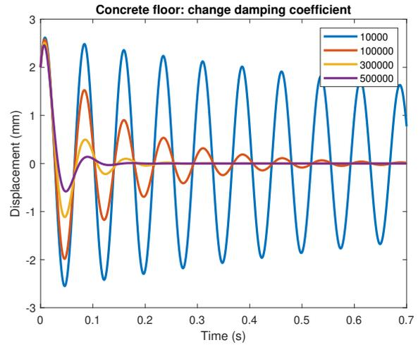
**Figure 4: Changing the damping coefficient of the concrete floor.**
