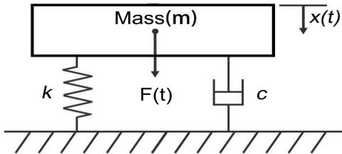
**Figure 1: The prototypical single degree of freedom oscillator [5]. The structure be simplified as a signal degree of freedom oscillator, contains three components: mass, spring, and damper.**
