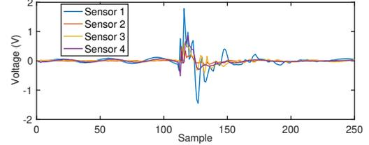
Fig. 4. Example signals of teeth contact-induced vibration.
