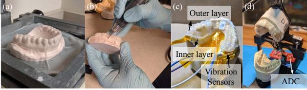
Fig. 2. TeethVib retainer-formed sensor building procedure.
